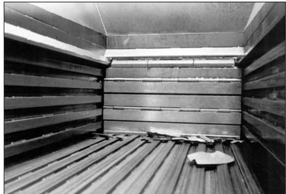
A bar grate system helps to keep the metal clips from working their way around the ram and interfering with ram movement. The pinning tunnels attached to the ram face allow the operator to pin the load in the container to reduce material fall-out when the container is pulled away from the compactor.
