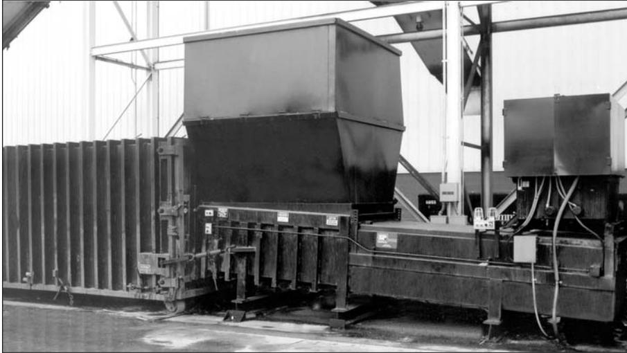
This CP-6002-D, six cubic yard capacity stationary compactor, is one of two machines used at this production plant to compact metal clips for transportation to a recycling facility.
