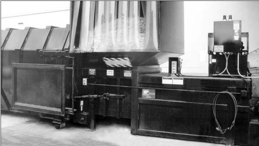
This CP-3002, three cubic yard capacity stationary compactor, is one of two machines used at Balimoy to collect cutting fluids from metal turnings and to compact the turnings for transportation to a recycling facility.
