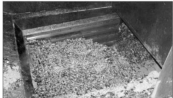
Metal turnings are loaded in the compaction chamber, then packed into the container. Fluid drains from the turnings during compaction and while held in the container prior to transportation.
