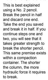
Now, back to our compactor. Without sufficient forces to break these shorter columns, it is very difficult to fill a container with as much material as possible. This is why SP Industries recommends dual cylinder compactors that create more packing
