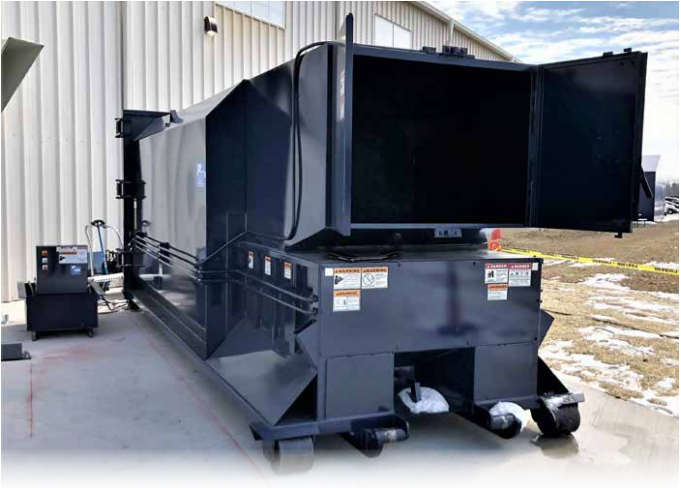
SCS2235 self contained unit with rear load ground load barn door style hopper with two interlocks.
