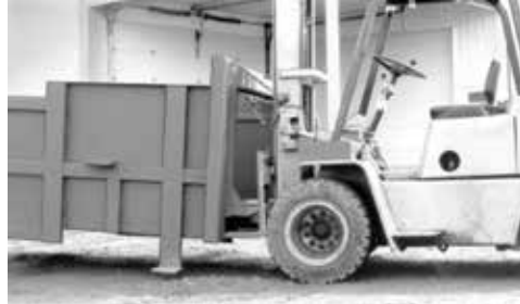
Lifting from the chamber end
