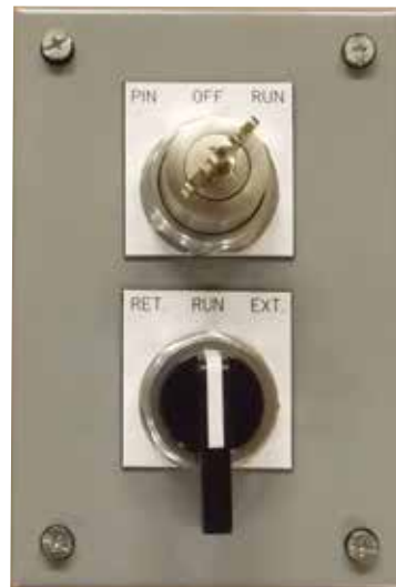
Pinning/Boost Override System Controls (mounted on the side of the pre-crusher/compactor)
