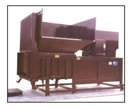
Loading hoppers direct material flow into the dewatering chamber.
