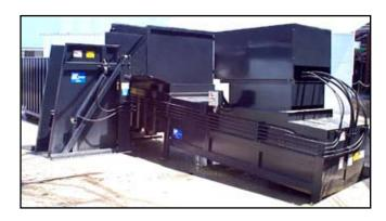
Dewatering precrushers can incorporate a variety of loading systems from hydraulic container dumpers, as shown in the photo, to conveyors that simplify material loading, improve flow, and increase volume throughput.
